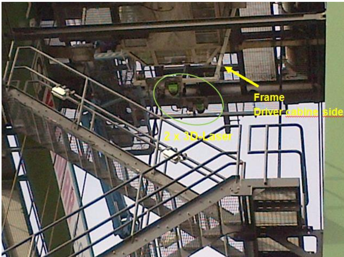
Figure 5: 2 x 3D-Laser scanner on the trolley (they are installed in different heights)
