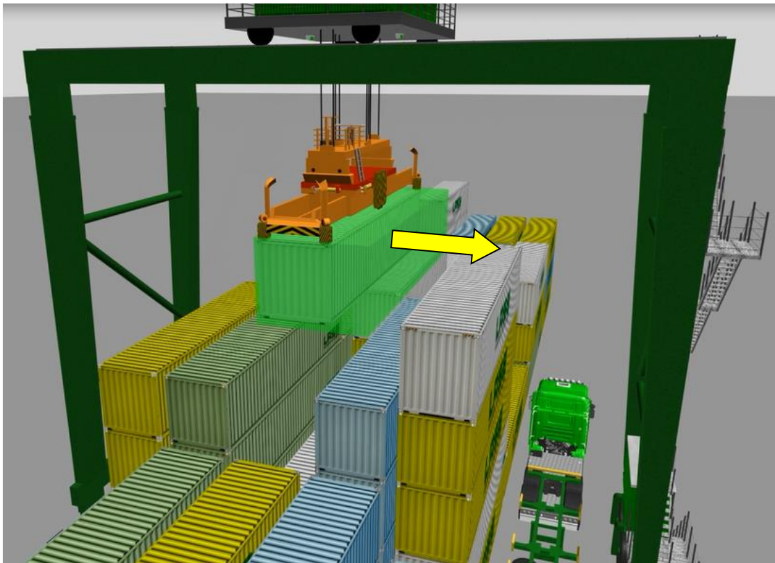
Figure 10: Surveillance Cube – trolley moves to the right
